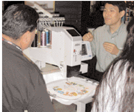
● Inbro spent seven years developing a self-threading, multicolor, single-needle embroidery machine.
