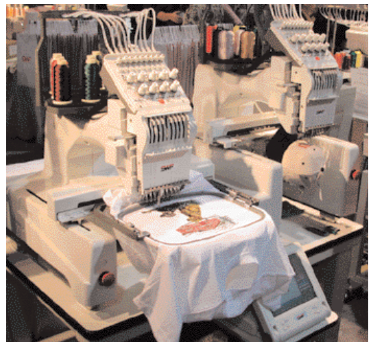
● SWF showed a prototype 2-head machine that can simultaneously embroider different items or different designs on each head.
