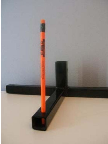
Mark the Holes
